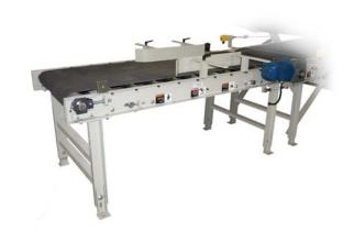
The Hamer Model 4100 In-Feed Bag Conveyor is a 24" wide, heavy-duty belt over roller style conveyor with a 10-gauge 6" formed channel side frame, with 1.9"x16 gauge steel bed rollers on 6" centers, and a 4" drive/tail pulley. The Model 4100 has a belt speed of 105 feet per minute and a 3/4 HP, TEFC motor. All 4100 series conveyors include bag guides. Powder coated.
