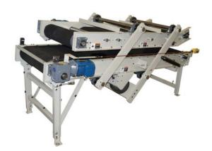
The Hamer Model 5100 Bag Flattening Conveyor is perfect for hand palletizing operations with a wide variety of bag sizes and products. This 24" wide incline conveyor with an adjustable 24" flattening conveyor mounted over top, is for bags 24" wide and up to 10" in thickness. It evenly disperses product inside the bag to improve bag handling and pallet build. Operators remove flattened bags from stacking table and build a level, even pallet. Can be used with manual or automated bagging systems.
